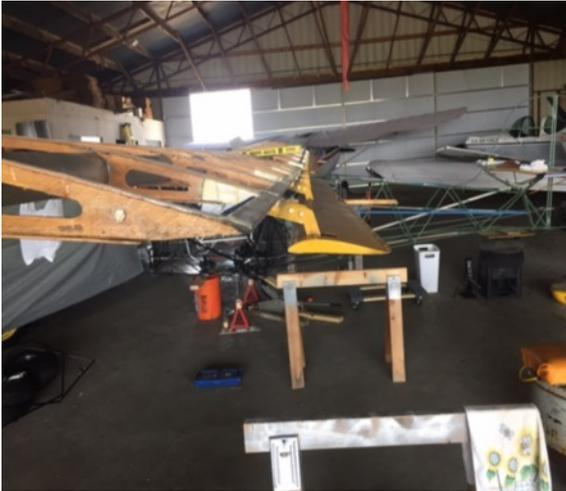
**Here is a shot of left wing flaperon in position and ready to be joined up with it's controls. The right side is in correct position to be joined up and holes drilled for second bolts in ribs. We are hoping to start covering next month.**
